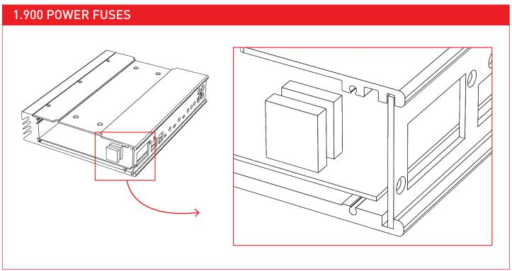
→ **TO USE:** Remove the end panel by the power terminals 2 x 25 amp ATC fuse
